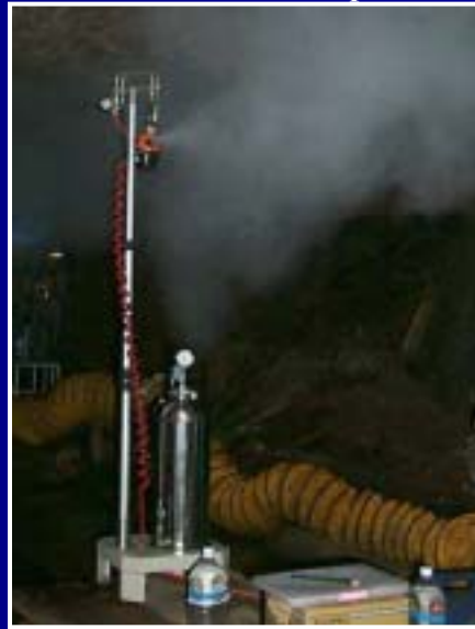
Spray device put in the bottom of shaft to supply aerosols
