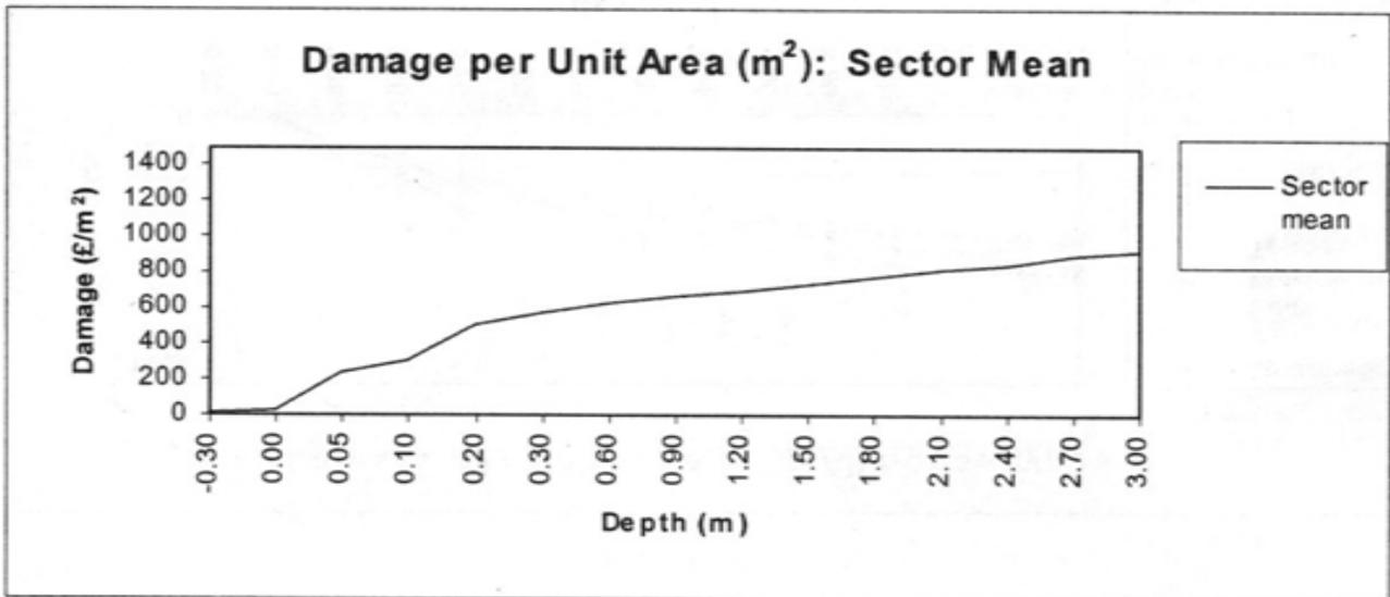
Figure 3: Depth-Damage relationship used for West Garforth
